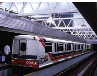
Figure 5. The skytrain in Vancouver, BC uses 0.30 kWh of energy per passenger-mile (given observed vehicle occupancy).
