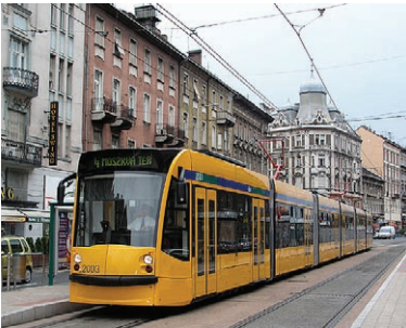
Figure 3. The modern Combino tram uses 0.11 kWh of energy per passenger mile (given observed vehicle occupancy).
