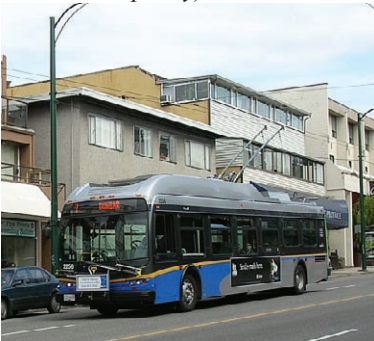
Figure 4. A trolleybus in Vancouver, BC is powered by overhead electrical wires therefore eliminating any tailpipe emissions. A trolleybus uses 0.36 kWh of energy per passenger mile (given observed vehicle occupancy).
